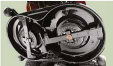
Cutting deck with two blades
